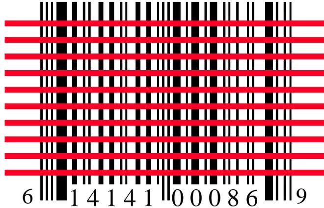
Figure 17 - Ten scan paths for vertical redundancy
